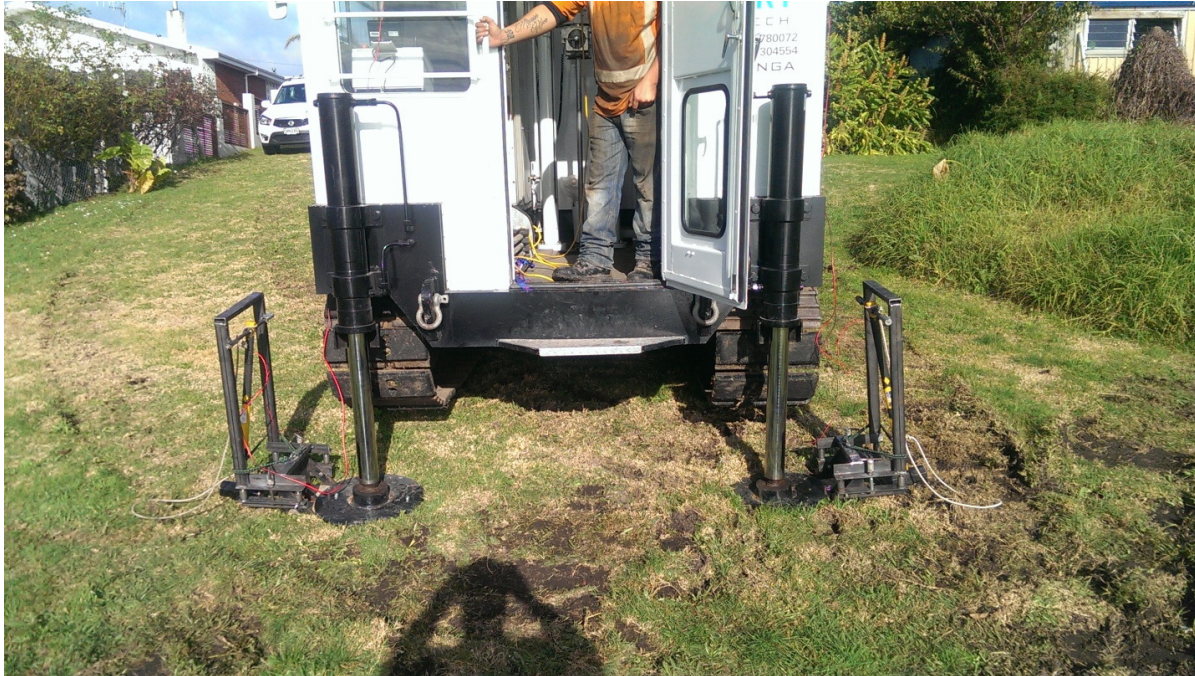
Figure 20: Perry Geotech Ltd. of Tauranga New Zealand SCPT site setup. The LS and RS SH source wave pendulum hammers which have a radial offset of 2.3 m from the downhole seismic probe are illustrated.
