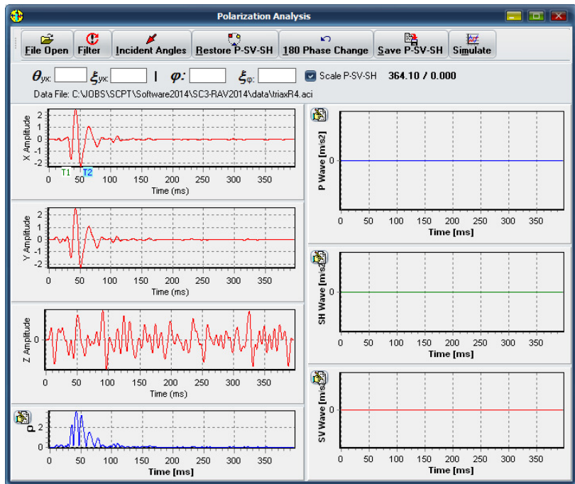
Figure 2. X, Y and Z axis seismic recordings from a SH SCPT investigation. Specification of time window T1 and T2 so that hodograms can be calculated.
