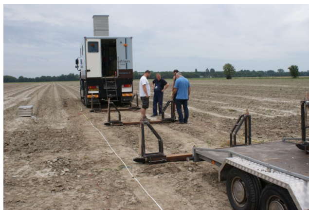
Figure 4. Wiertsema & Partners of The Netherlands SCTT-NMO-SCPT site setup. SH pendulum hammer beam sources have sensor-sensor offsets of 1.85m, 5m and 10m.
